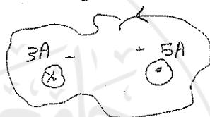
32- The circuit shown is in a uniform magnetic field that is into the page and is decreasing in magnitude at the rate 152 T/s. The current in the circuit (in Amperes) is:
